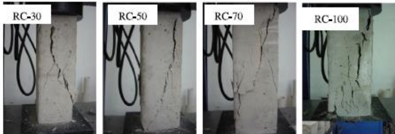
(a) Failure process of recycled aggregate concrete prisms
